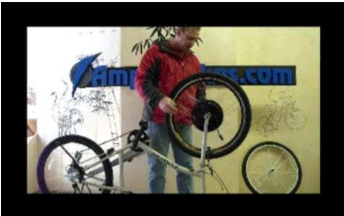
If you have a **disk brake** remove it from your bike and install it on the hub motor before installing the wheel using the screws on the motor. Note: **You cannot install ANY hub motor**
