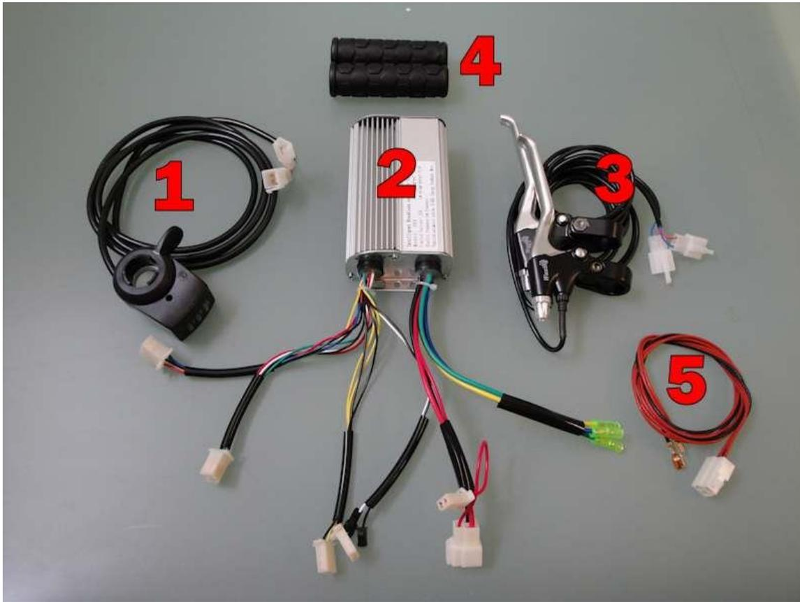
1 Thumb Throttle. (We have changed the design to a newer thumb throttle shown here.)
